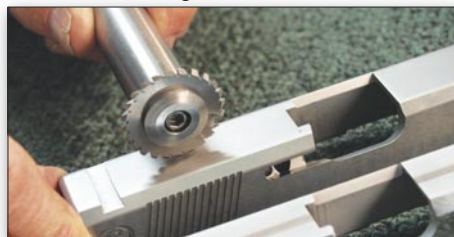
Showing cutting position for sight track
