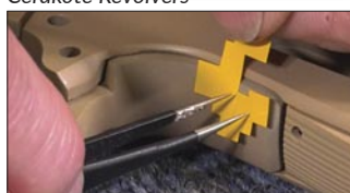
Applying a Stencil
