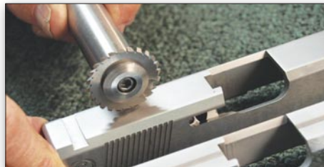
Showing cutting position for sight track
