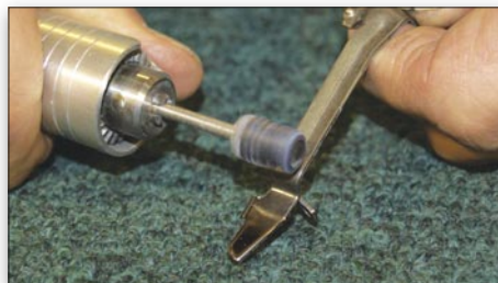
Doing a trigger job, smooth and tune
